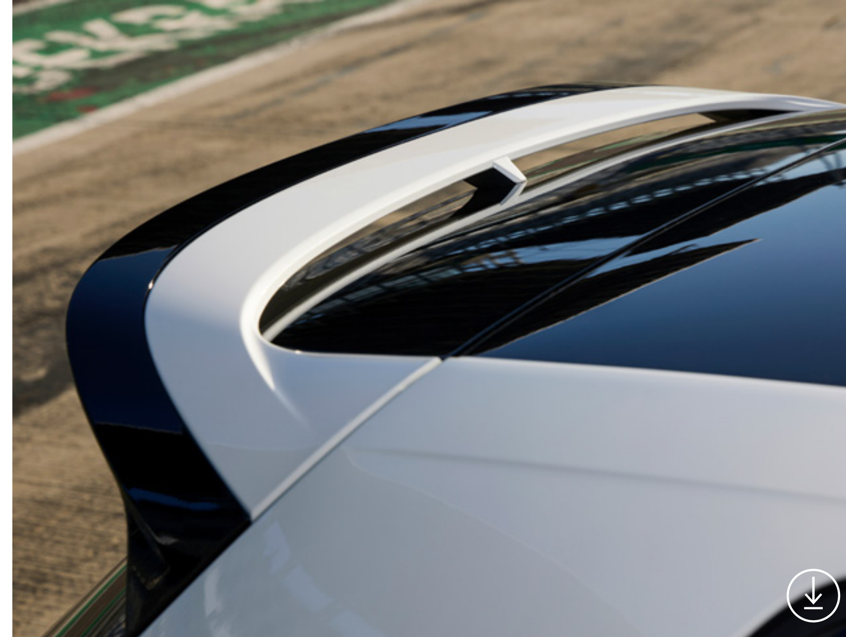
The Golf GTI Clubsport's distinctive roof spoiler provides additional downforce on the rear axle
