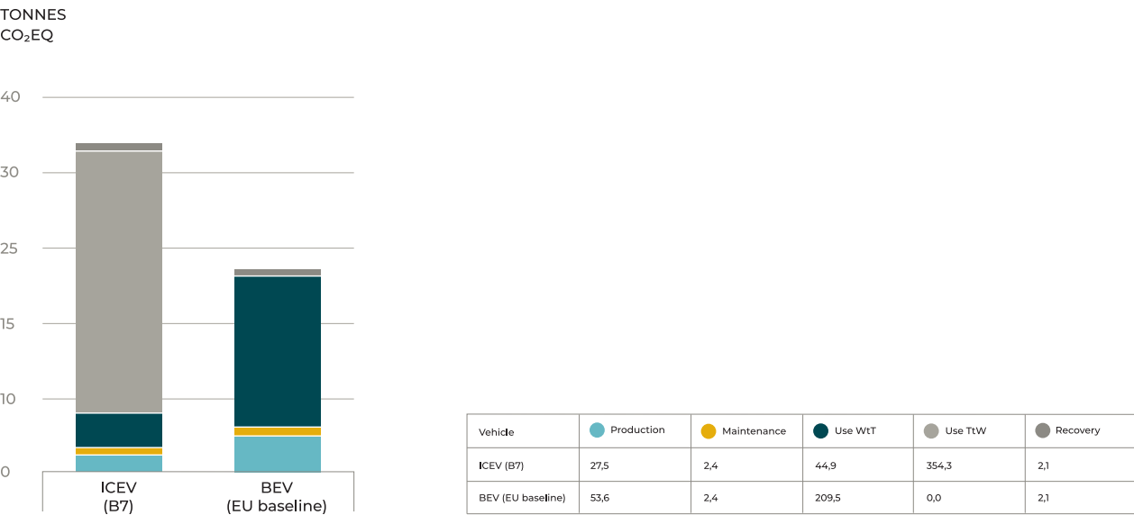
Figure 19: Total lifecycle carbon-dioxide emissions presented per lifecycle phase. The use phase is divided into WtT (Well to Tank) and TtW (Tank to Wheel)
