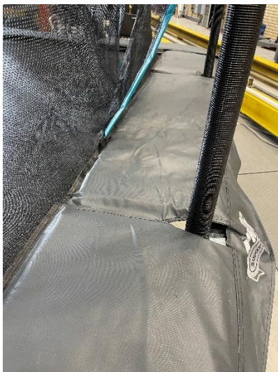
Picture 24 Small holes at the poles and frame exposed (Jump King)
