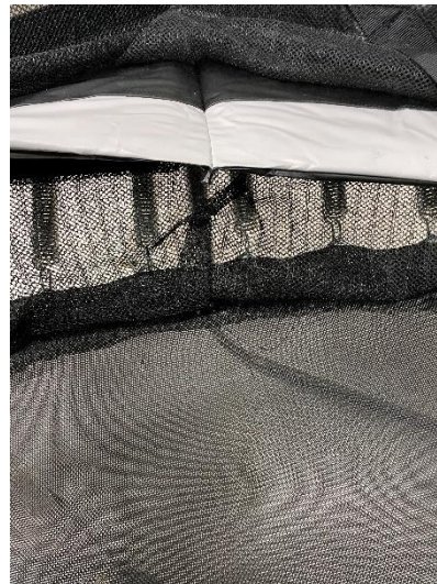
Picture 20 Full coverage of springs and net stitched to padding (North 500)
