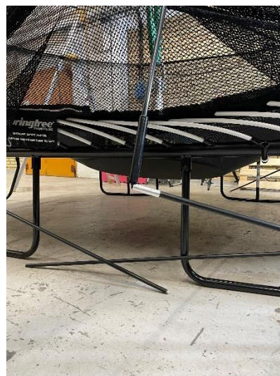
Picture 35 500kg at the side (Springfree)
