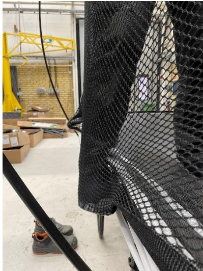
Picture 21 Entrapment risk on the side (Springfree)
