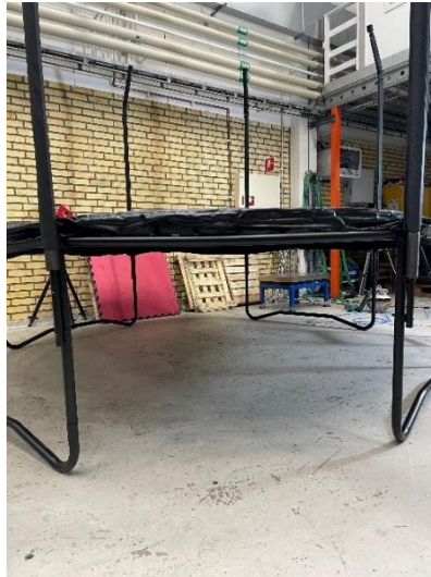
Picture 27 Frame tube a little bent (Salta)
