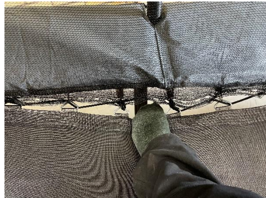
Picture 18 Gap between the stitches, entrapment risk (Jump King)
